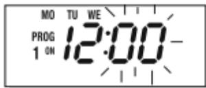
• Press the right arrow button '→' to select the minutes (in this case 10). Press the 'SET' button to save, and 'Prog 1 ON' will start to flash.
