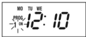
• Press the right arrow button '→' to change the 'Prog 1 ON' to 'Prog 1 OFF'. Press the 'SET' button to save, and the days/day groups will start to flash.
